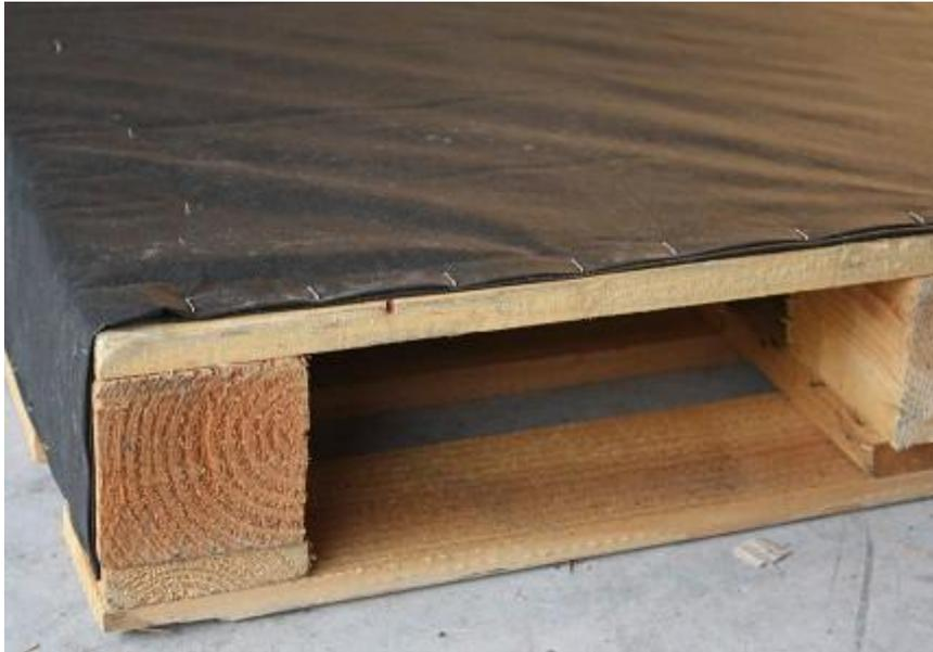
Hold the two pieces of landscape fabric together as if they were one piece of fabric. Fold over the top edge by one inch and center it on the top board of the back of the pallet. **Staple the fabric into place near the top edge of the top board.** Smooth the fabric out to the left and right and
